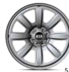
5. Steel wheel 17". 17" eight-spoke steel wheel, anthracite, 6.5Jx17, suitable for 205/55 R17 tyres. Ideal for winter tyre use. Cap included, nuts not included. H8401ADE50
