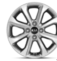
3. Alloy wheel kit 17", type-B. 17" eight-spoke alloy wheel, 6.5Jx17, suitable for 205/55 R17 tyres. Kit includes a cap and four nuts. H8F40AK400
