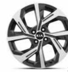
1. Alloy wheel kit 16", type-C. 16" four double-spoke alloy wheel, 6.0Jx16, suitable for 195/55 R16 tyres. Kit includes a cap and four nuts. H8F40AK120
