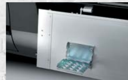
INTERNAL STEPS FOLDING INTO SIDEBOARDS
