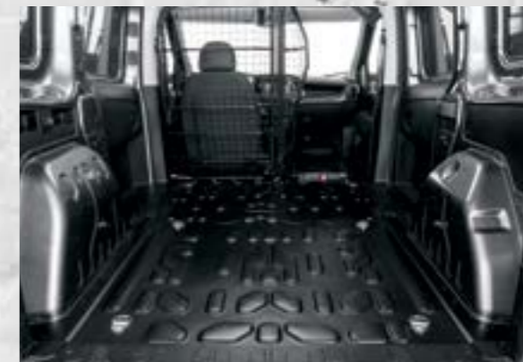
Swivel partition, available for 2 seats configuration only
