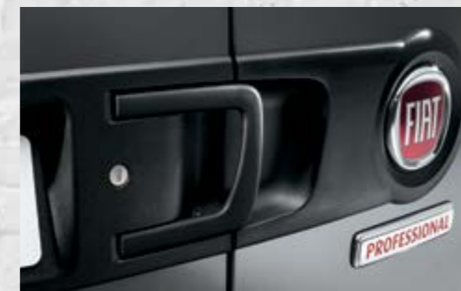
REAR WING DOOR HANDLE WHICH IS EASY TO OPEN, EVEN WITH A SINGLE FINGER
